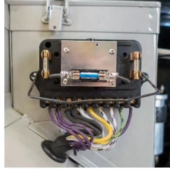
RF91 converted to solid state
