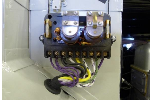
RF91 voltage regulator (original solenoids)
