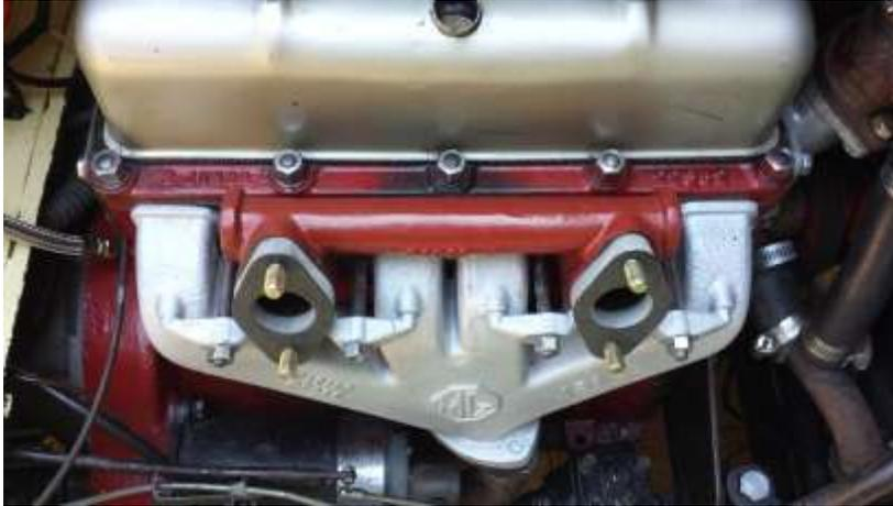
The new fuel hoses and heat shield arrived in the post within a few days of each other so all parts were removed and numerous applications of carburetor cleaner were applied. The old carburetors were black with grime and would not be fair to the maker of the heat shield to have them beside such a gleaming shiny product.
