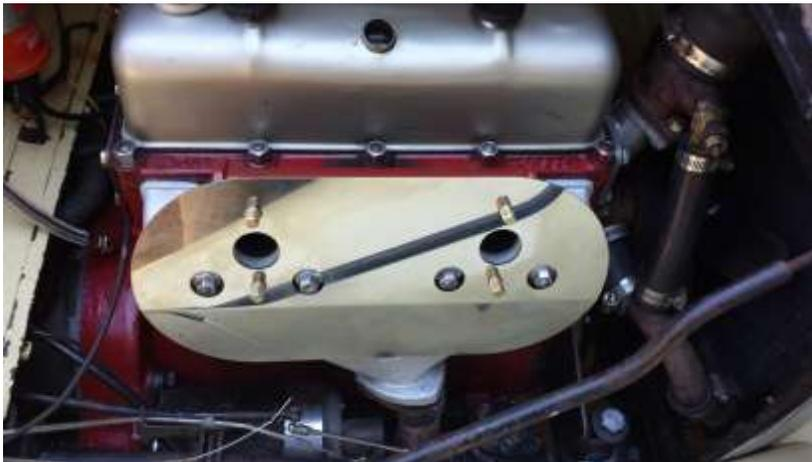
I have not had the chance yet to see if the vapor lock is cured but discovered that the linkage between was not balanced and on listening to each carburetor at idle with air filter off could hear suction was different, this has been rectified and car now has a steady idle.
