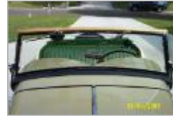
18 Test fitting top bow wood
