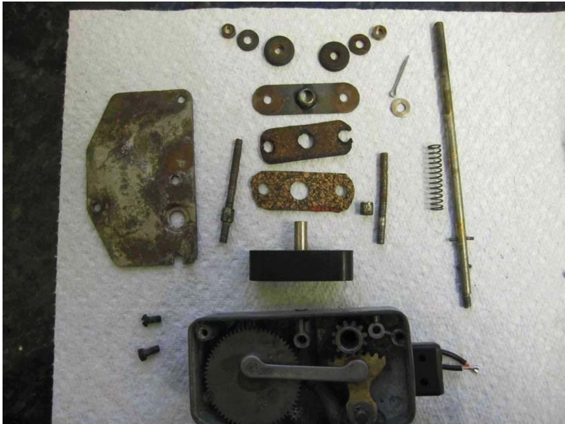
Photo 4 – Exploded view of Front (Gearbox side)
